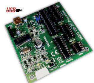
This PICKit™2 Development Programmer is very versatile. It features on board sockets for many types of PIC® microcontrollers. Also provided is an ICSP connector, to program your onboard device. It is compatible with the free tools from Microchip such as the MPLAB® IDE environment.
